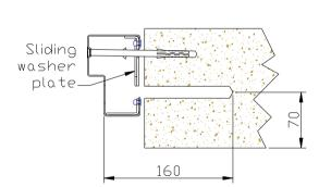
10. Ensuring that the sliding washer plate is away from, and not covering the 16mm frame tray holes, drill through the access holes in face 2 with a 15mm masonry bit to a depth of 160mm.
